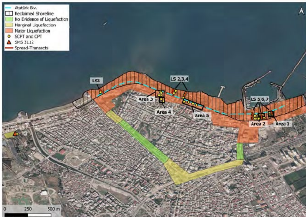
Figure 2- 17 Overview of liquefaction observations and study areas within Iskenderun (from Moug et al., 2024).
