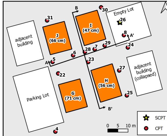
Figure 2-19 Overview of Area 1, note that the numbers inside the buildings show the settlements measured by Moug et al. (2024).
